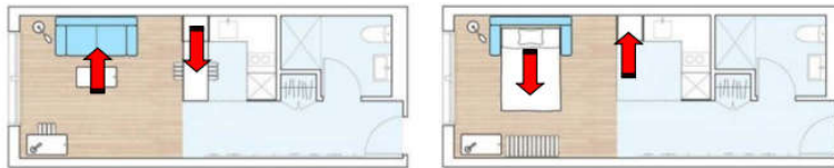
Figure (17) depicts a limited-space apartment that includes multifunctional pieces of furniture (Canepa, 2017, p. 5).
