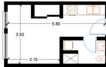
Figure (1) illustrates the adoption of an open plan to enhance flexibility in a space-limited apartment, with an area of 20.3 m 2 , (Husein, 2021, p. 4)
