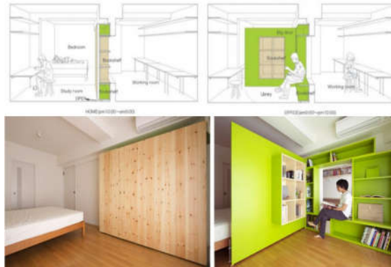
Figure (5) Shows partition that can rotate at a specific angle (90 degree), (Kavut, 2020, p. 148).
