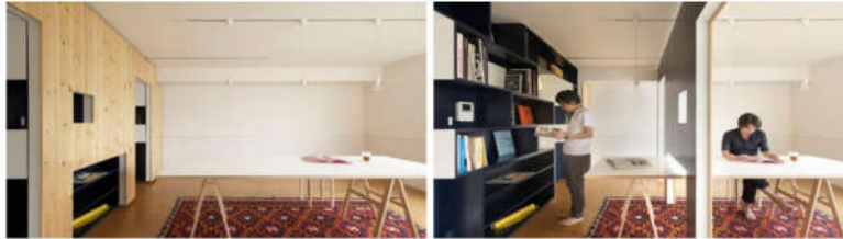
Figure (4) illustrates a movable partition that divides space and boots its flexibility (Kavut, 2020, p. 148).
