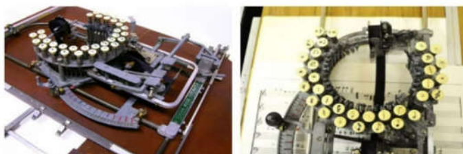
Fig. (2): (Keaton) Typewriting Machine; developed and consists of 33 buttons or keys, designed by Robert H Keaton in 1955
