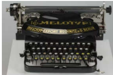
Figure (1): Melotyp Typewriter specially designed for musical notation. Manufactured in Arko Factory in Frankfurt in 1936.
